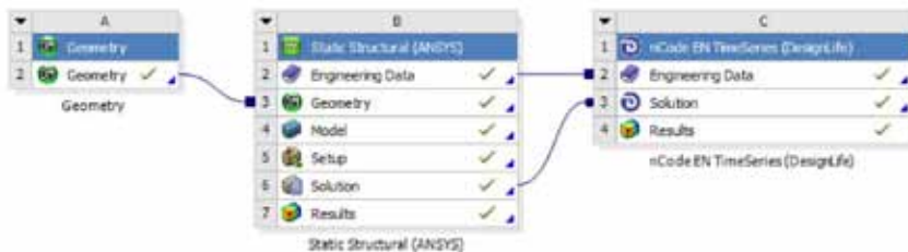
Fatigue life simulation based on static FE results and cyclic loadings
