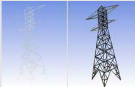
Simplified beam model representing an electrical tower
