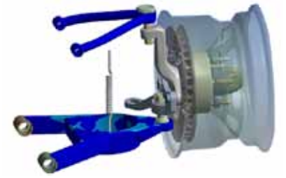
Transient analysis of rigid/flexible suspension mechanism using kinematic joints, springs and contacts
