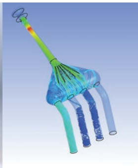
▲ Air box CAD model (left), 3-D CFD simulation (center), air box installed in racing car (right)
