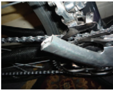
Bicycle crank fatigue failure from cyclic loading
