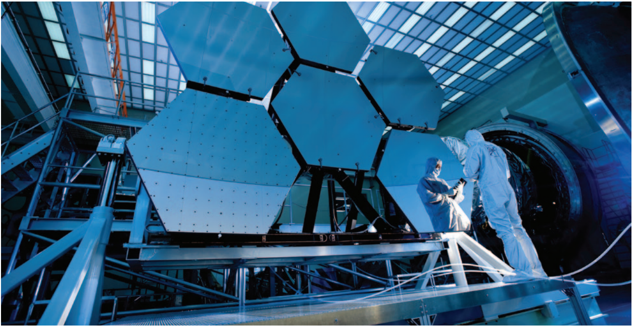
Six of the 18 mirror segments ready for optical test in a cryogenic environment at NASA Marshall Space Flight Center
